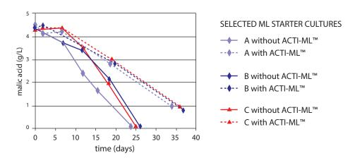
Kinetics of malic acid degradation in a Chardonnay wine (alcohol 14,1% vol, T-SO<sub>2</sub> 14, ppm pH 3,3) after direct inoculation with selected ML starter cultures with and without addition of ACTI-ML™.
